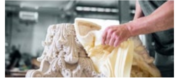
Cast stone is a suitable alternative to historic carved stone that cannot be repaired or replaced. Image courtesy of Had-donstone.
