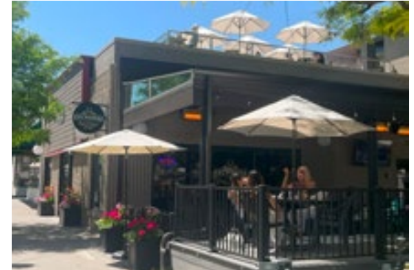
The rooftop patio on this non-historic building in the historic district is set back from the primary and secondary facades, ensuring that the rooftop patio is minimally visible from the public right-of-way. Photo by KDG, 2023.
