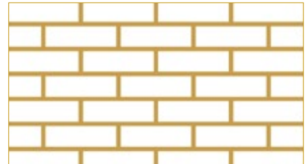
Mortar joints, shown in yellow, are appropriate places to install signage anchoring. It is not appropriate to anchor signage through masonry faces, shown in white. Diagram by KDG, 2023.
