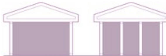
At left, it looks as if the columns would not support the pediment, and as if it might sag in the middle. Diagram by Architects Four, Inc., 1999, redrawn by KDG, 2023.
