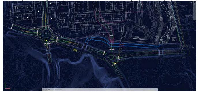
I was having fun with roundabout geometry, playing with bicycle bypass best practices at Center and going for KISS at Hines. On a page width view you can see the existing roadways, the Ski Jump Hill terrain, and the Johnson Creek Bridglets as they define the geometry. A strong S-Curve was needed to line up with Hutton. The double-arrow shows a small shift to New Griswold that works better for all.
